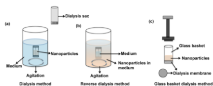
Fig. 1. Schematic representation of dialysis methods. (a) dialysis sac method, the nanoparticulate systems are placed inside the dialysis sacs; (b) reverse dialysis sac method, the nanoparticulate systems are added to the medium outside the dialysis sacs and the inside medium is analyzed for released drug at different time intervals; and (c) glass basket dialysis method, a glass cylinder with its bottom sealed by a dialysis membrane is used.
