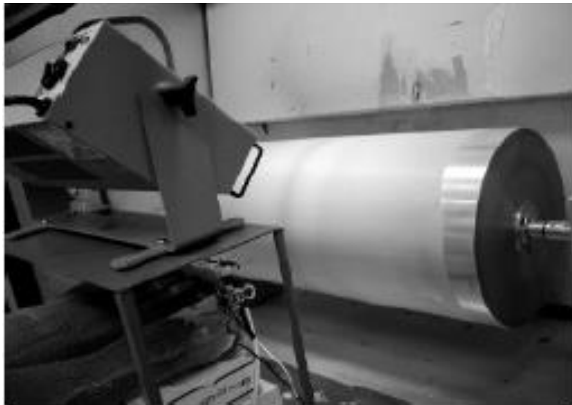
Figure 2 Production of a nanofiber fabric on a rotating collector drum with three electrospinning nozzles (hypodermic needle spinnerets).
